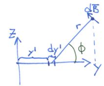
$$B_z = -\frac{\mu_0 J_{s0}}{2\pi} \int_0^w dy' \frac{(y-y')}{r^2} = -\frac{\mu_0 J_{s0}}{2\pi} \int_0^w dy' \frac{(y-y')}{(y-y')^2 + z^2}$$
