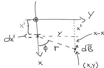
$$\begin{aligned}\hat{a}_\phi &= (-\hat{a}_x \sin \phi + \hat{a}_y \cos \phi) \\ &= (-\hat{a}_x \frac{y}{r} + \hat{a}_y \frac{(x-x')}{r}) \\ r &= \sqrt{(x-x')^2 + y^2}\end{aligned}$$
