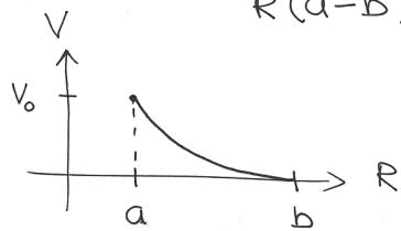
$$\begin{aligned} \bar{E} &= -\nabla V = -\hat{A}_R \frac{\partial V}{\partial R} \\ &= -\frac{abV_0}{R^2(a-b)} \hat{A}_R \\ &= \frac{abV_0}{R^2(b-a)} \hat{A}_R \end{aligned}$$
