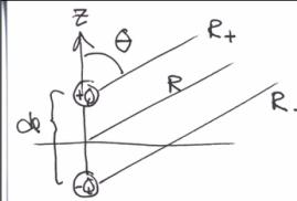
$$\rightarrow V = \frac{Q}{4\pi\epsilon_0} \left\{ \frac{e^{-i\beta R_+}}{R_+} - \frac{e^{-i\beta R_-}}{R_-} \right\}$$
