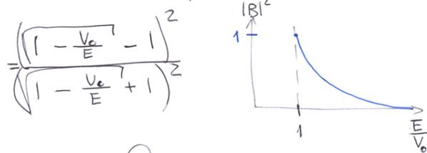
$$T = 4 \frac{\sqrt{(E - V_0)E}}{(E' + \sqrt{E - V_0})^2} = \frac{4 \sqrt{(1 - \frac{V_0}{E})}}{\left( \sqrt{1 - \frac{V_0}{E}} + 1 \right)^2}$$
