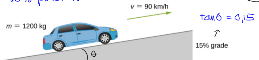
Figure 7.15 We want to calculate the power needed to move a car up a hill at constant speed.
