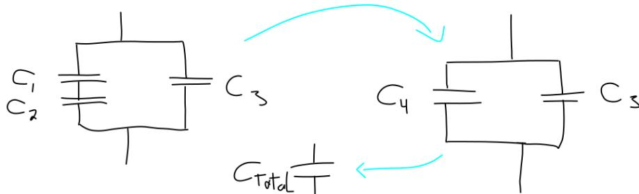
$$\frac{1}{C_4} = \frac{1}{C_1} + \frac{1}{C_2} \rightarrow C_4 = \frac{1}{\frac{1}{C_1} + \frac{1}{C_2}}$$
