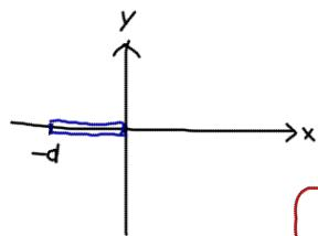
$$\Phi(\bar{r}) = -G \int_{-d}^{\frac{d}{2}} dr' \frac{g(\bar{r}')}{|\bar{r} - \bar{r}'|}, \quad g = \frac{M}{d}$$
