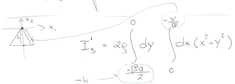
$$= 2g \int_{-\frac{\sqrt{3}a}{2}}^{\frac{\sqrt{3}a}{2}} dy \left\{ \left( \frac{x^3}{3} + xy^2 \right) \right\}_{0}^{\frac{y}{\sqrt{3}}} = -2g \int_{-\frac{\sqrt{3}a}{2}}^{\frac{\sqrt{3}a}{2}} dy \left\{ \frac{y^3}{3(\sqrt{3})^3} + \frac{y^3}{\sqrt{3}} \right\}$$
