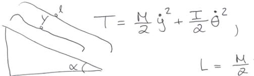
$$T = \frac{M}{2} \dot{y}^2 + \frac{I}{2} \dot{\theta}^2, \quad U = Mg(l-y)\sin\alpha, \quad y=R\theta$$
