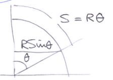
$$\Delta L = \omega_y R \sin \theta \cdot T = \omega_y R \sin \left( \frac{S}{R} \right) \frac{S}{v}$$
